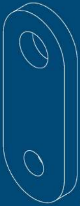
KTTFP000110 Top Fixing Plate (146 × 56 mm; Ø26 + Ø18 holes)
